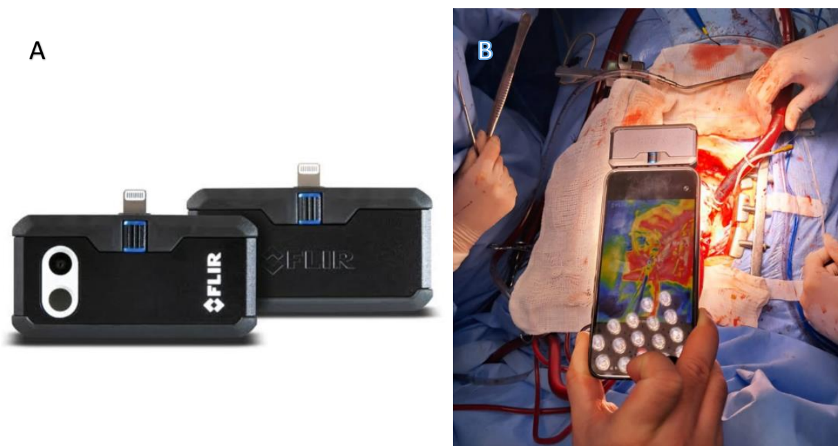
Fig. 1 - A) and B) Portable thermal camera (FLIR One Pro) attached to a smartphone, used for intraoperative acquisition of thermographic images at approximately 30 cm from the surgical field.
